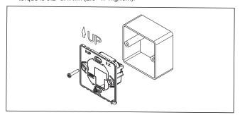
4) Re-mount the front cover via snap-fit connection.
